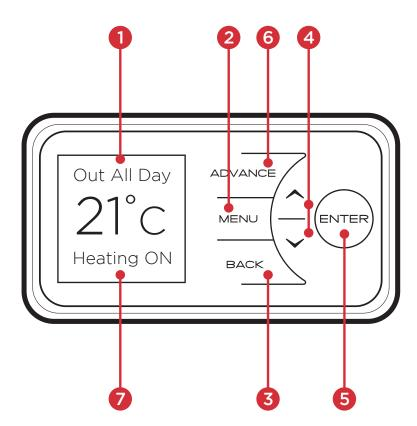
The heater is fitted with an adjustable thermostat enabling the room temperature to be controlled. The minimum room temperature is 7°C. The maximum temperature is set to 30°C. A temperature of 21°C is a common comfortable room temperature.
