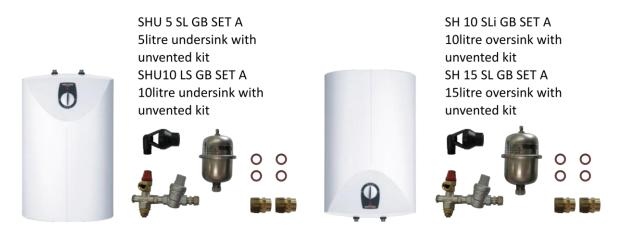
These water heaters come supplied complete with a pressure reducing valve, in-line strainer non-return valve, pressure relief valve, two reducers, expansion vessel, two connection pieces, four washers and a tundish. These can be connected directly to the mains cold water supply - see following digram.
