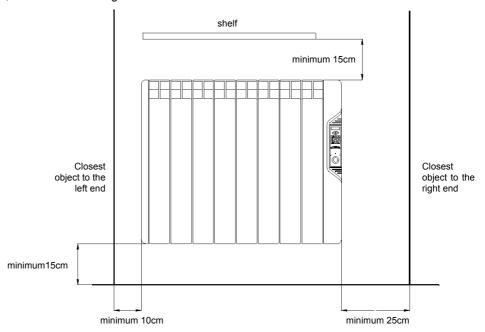
Position and fix the brackets at the correct distance from the floor and hang the unit on the hooks of the brackets. and mark the wall. Use the polystyrene packaging to level the heater and protect the floor. Use the heater as a template and mark the fixing points on the wall using a pencil through the two fixing holes in the square brackets.
